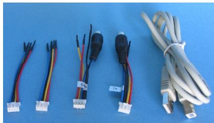
Pass through power & video cables.
